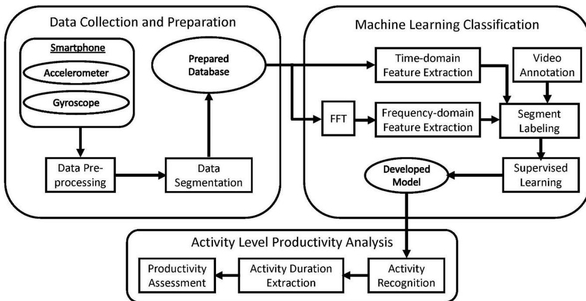
Figure 1. Components of the developed framework
