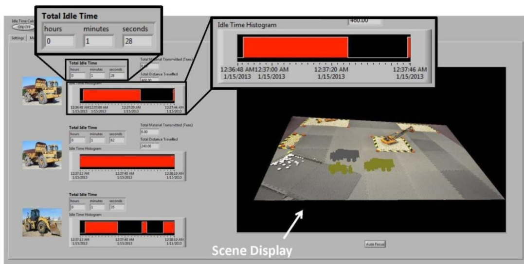
Figure 3. Snapshot of the developed GUI for equipment idle time analysis.
